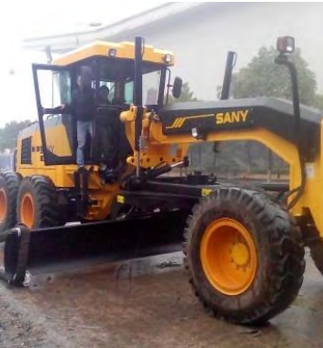
SMG200 Motor Grader in Gradeability Test
