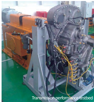
Transmission performance testbed
