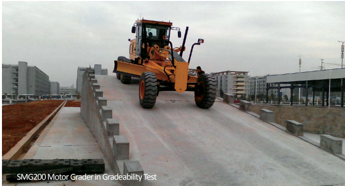
SMG200 Motor Grader in Gradeability Test
