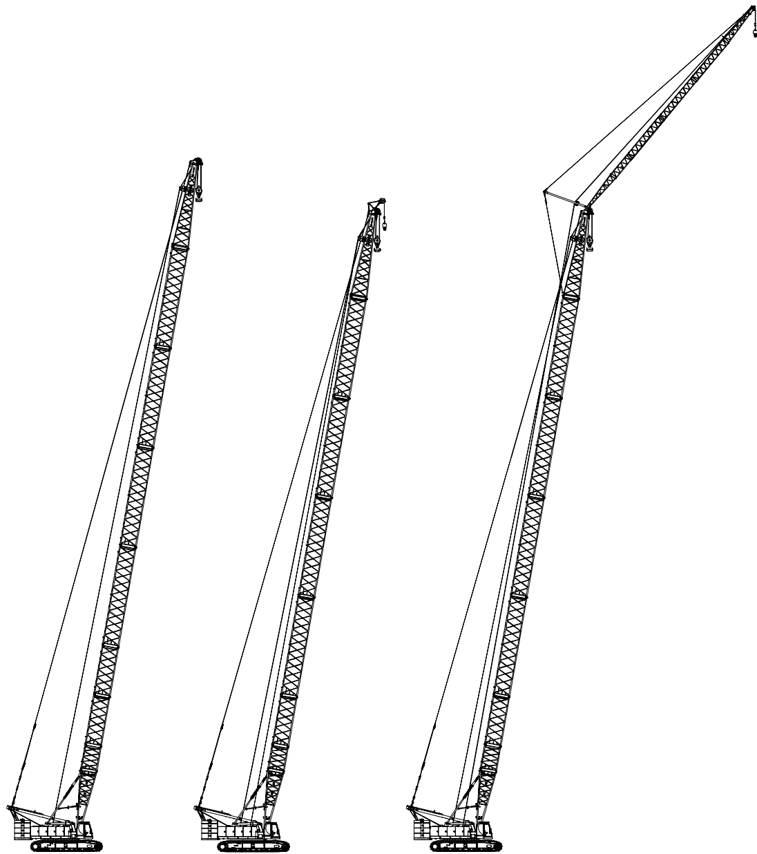
Operating condition of light-duty boom H L (18~81)m (53+16)t
