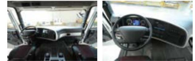
The four point shock absorbing mounting, double layer door sealing, and noise reduction technology built into the cab help reduce driver fatigue during those long days on the job. The interior trim of red and black exudes a sports car feeling to reduce visual monotony. Bluetooth technology with steering wheel controls allows hands free use of mobile devices (where permitted) to maintain contact with coworkers.
