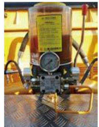
Semi-auto lubricating grease pump
