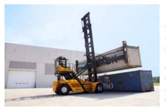
The load-sensing hydraulic system calculates the exact power needed for quick, smooth operation. SANY's fast-activating locking mechanism and torsion-resistant frame help the machine efficiently lift and stack 20- to 40-foot containers with precision. Anti-jamming features
