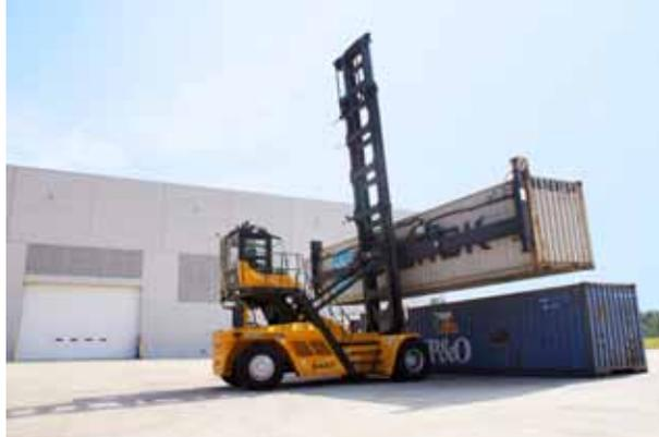
The load-sensing hydraulic system calculates the exact power needed for quick, smooth operation. SANY's fast-activating locking mechanism and torsion-resistant frame help the machine efficiently lift and stack 20- to 40-foot containers with precision.
